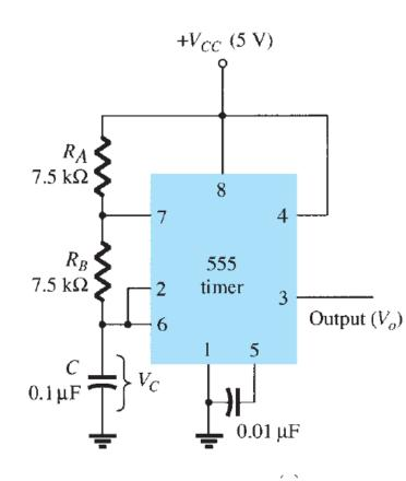
$$T_{\text{high}} \approx 0.7(R_A + R_B)C$$
