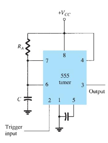
• When trigger input signal goes negative, it triggers the one-shot, with output at pin 3 then going high for a time period given by
