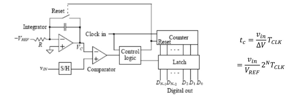
ΔV the smallest change in analog signal that will result in a change in the digital output, also called «Resolution»
